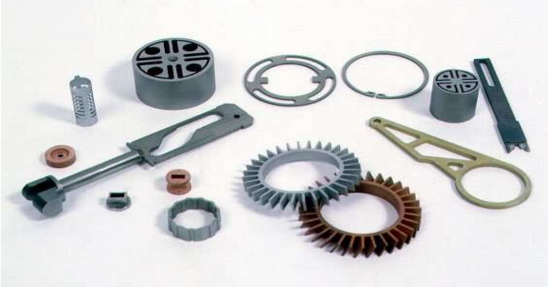
Figure 14: Difficult internal parts made by EDM process
